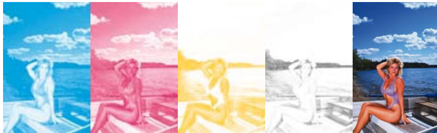
Process Separations, from l - r: Cyan, Magenta, Yellow, Black, and Composed
